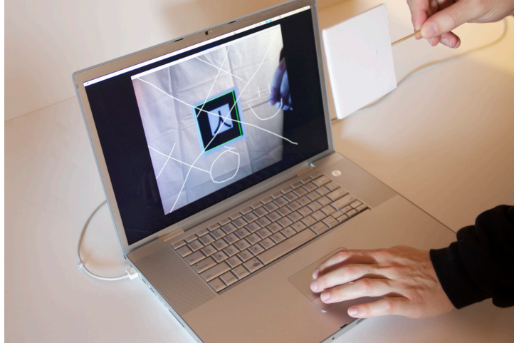
Figure 4: Finger Paint application running on Mac OS X. Drawing is done using the track pad.
